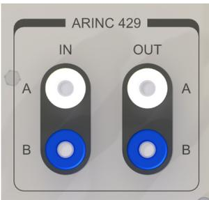
Connect the test clip leads to the ARINC 429 source. Ensure that the red test clip is connected to the ARINC 429 "A" source and the black test clip is connected to the ARINC 429 "B" source.
